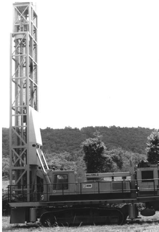
Fig. 13.15 Track-mounted rotary drill with air compressor. (Caterpillar Tractor Co.)
